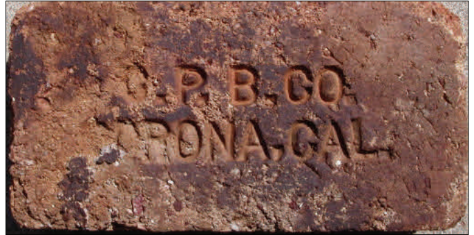
View of the marked face of the Corona wire-cut firebrick. Contributed Jack Bower.
